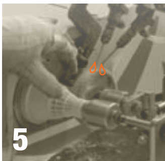
5 Klebmaschine zum Fixieren des Doppelgarns. Gluing machine to fix the double-yarn.
